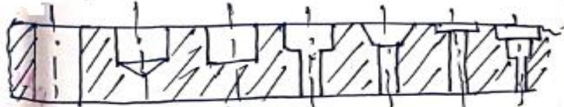
Through hole, Blind hole, Blind hole with flat bottom, Counter hole, Counter sink hole, Spot face, Step die.
