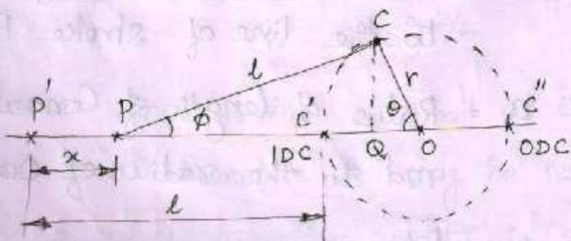
Consider the motion of a Crank and Connecting rod of a reciprocating steam engine as shown in fig. Let OC be the Crank and PC the Connecting rod.
